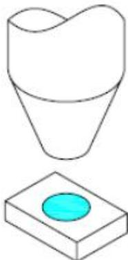
Outer diameter of collet should be larger than the lighting area
